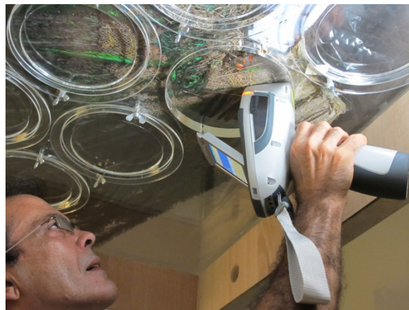
Fig. 2. Dr. Roman Padilla-Alvarez (IAEA) performing handheld XRF analysis of the feather headdress lying horizontally on a specially constructed acrylic table.
